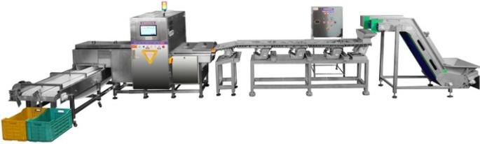
Highlights: Accuracy 95%; Throughput ITPH; Automated feeding and pneumatic rejection system; Safety: <math>\lt; 1\mu\text{Sv/h}</math>, Atomic Energy Regulatory Board (AERB) certified; Proven Reliability: 4+ years of use in production lines; Subsidy Eligibility: Recognized by APEDA.
